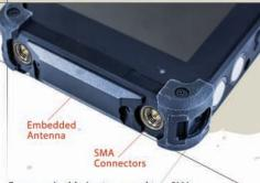
For an embedded antenna and two SMA connectors choose: WiFi, Bluetooth\*, WWAN or GPS
