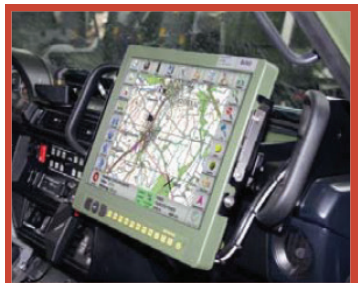
MOJAVE RD15 vehicle installation
